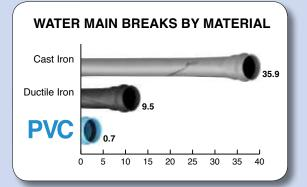
Further, a study by the Los Angeles Department of Water and Power determined corroded cast-iron pipe was overwhelmingly to blame for a rash of breaks in 2009.
