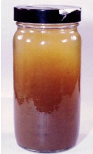
Discolored water from iron sediments re-suspended from mainflushing. Photo by John Marchand
